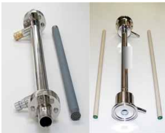
Fig. (3). Ceramic membranes and steel housings.
