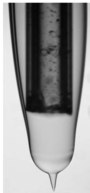
Fig. (3). A hollow quartz capillary with 170 \mu\text{m} outer diameter is inserted and centered into a Chiptip.
